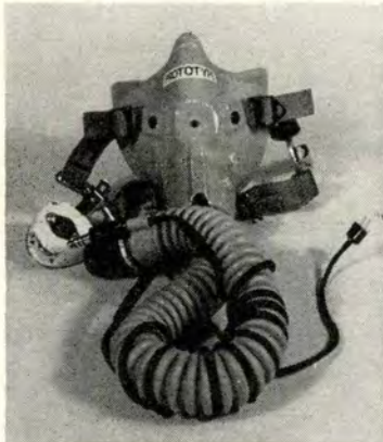
Prototype MBU-7/P oxygen mask. Improvements over MB-5/P include better retention under high G forces, reduced restriction to breathing. Mask is now in Operational Testing and Evaluation.
