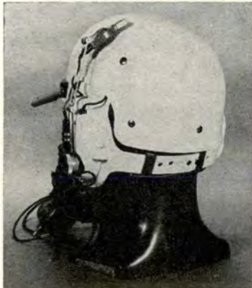
Proposed improvement to HGU-7/P helmet for non-ejection seat equipped aircraft. Helmet will improve headset suspension to provide more comfort. It has better visor and should fit better.
