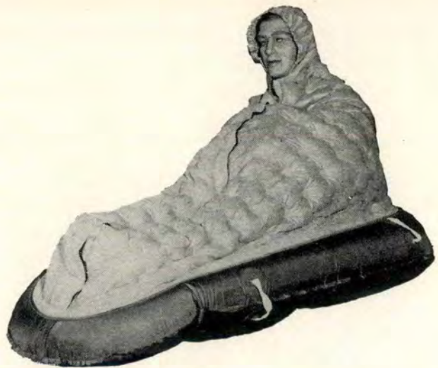
New insulated life raft described in story. Main features are easier access, greater protection. Raft increases survival time in cold water by factor of three.
